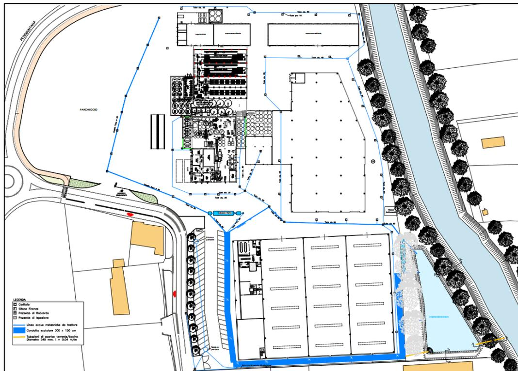
FIGURA 4-21. SCHEMA DELLA GESTIONE DEGLI SCARICHI IDRICI
