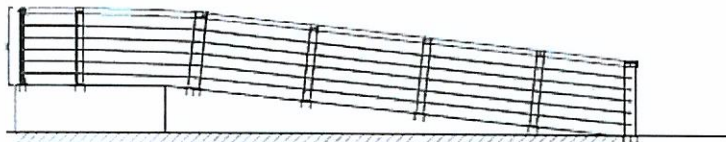
Ringhiera rampa ( Side View)
