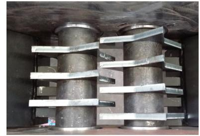
Bottle perforators used prior to bailing presses
