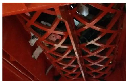
Discharge screen under the 4 shaft shredder
