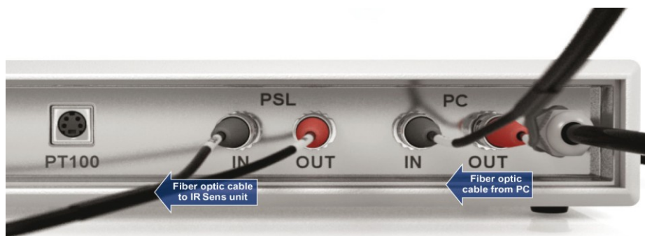
Figure 2 Fiber optic cable connections at the PT100 unit
