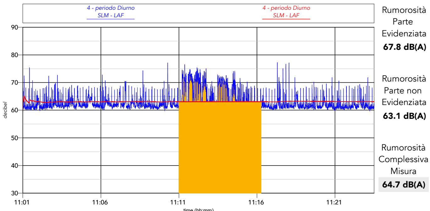
**Percentili complessivi:**  $L_1 = 73.3 \text{ dB(A)}$     $L_{10} = 68.1 \text{ dB(A)}$     $L_{50} = 61.9 \text{ dB(A)}$     $L_{90} = 60.8 \text{ dB(A)}$     $L_{95} = 60.6 \text{ dB(A)}$
