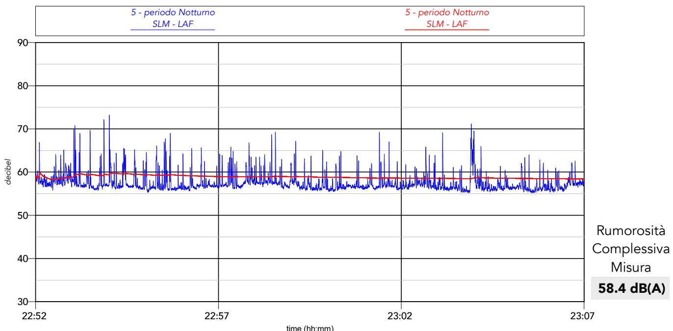
**Percentili complessivi:**  $L_1 = 66.1 \text{ dB(A)}$     $L_{10} = 60.3 \text{ dB(A)}$     $L_{50} = 56.9 \text{ dB(A)}$     $L_{90} = 56.0 \text{ dB(A)}$     $L_{95} = 55.8 \text{ dB(A)}$
