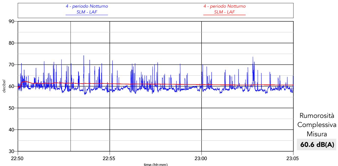
**Percentili complessivi:**  $L_1 = 68.7 \text{ dB(A)}$     $L_{10} = 62.6 \text{ dB(A)}$     $L_{50} = 59.0 \text{ dB(A)}$     $L_{90} = 58.0 \text{ dB(A)}$     $L_{95} = 57.6 \text{ dB(A)}$
