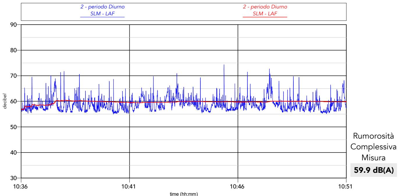
**Percentili complessivi:**  $L_1 = 67.8 \text{ dB(A)}$      $L_{10} = 62.1 \text{ dB(A)}$      $L_{50} = 58.2 \text{ dB(A)}$      $L_{90} = 56.2 \text{ dB(A)}$      $L_{95} = 55.9 \text{ dB(A)}$
