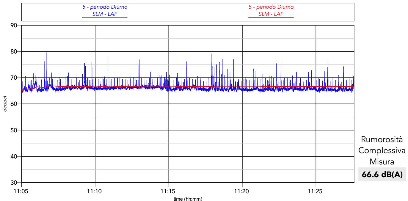
**Percentili complessivi:**  $L_1 = 72.3 \text{ dB(A)}$     $L_{10} = 67.6 \text{ dB(A)}$     $L_{50} = 65.9 \text{ dB(A)}$     $L_{90} = 65.2 \text{ dB(A)}$     $L_{95} = 65.0 \text{ dB(A)}$
