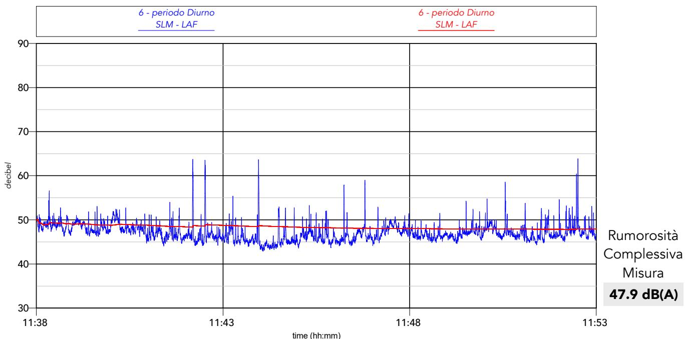
**Percentili complessivi:**  $L_1 = 53.2 \text{ dB(A)}$     $L_{10} = 49.5 \text{ dB(A)}$     $L_{50} = 46.8 \text{ dB(A)}$     $L_{90} = 45.0 \text{ dB(A)}$     $L_{95} = 44.6 \text{ dB(A)}$
