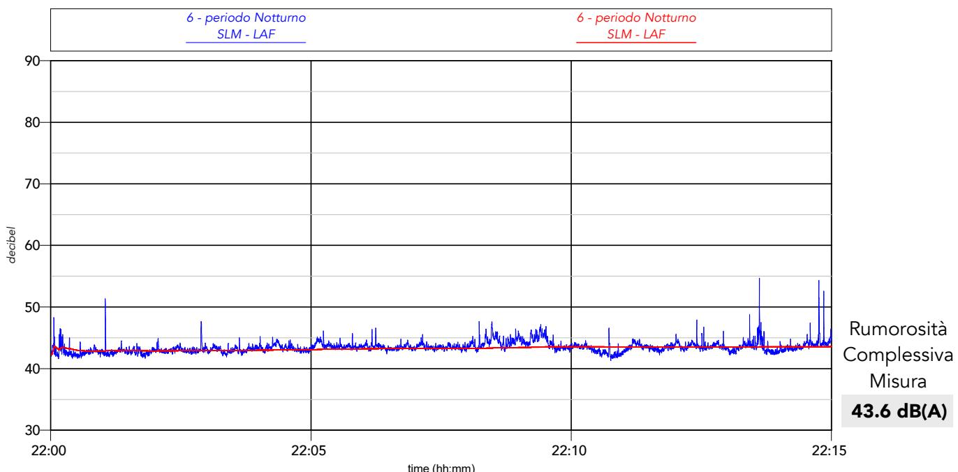
**Percentili complessivi:**  $L_1 = 46.3 \text{ dB(A)}$     $L_{10} = 44.4 \text{ dB(A)}$     $L_{50} = 43.4 \text{ dB(A)}$     $L_{90} = 42.6 \text{ dB(A)}$     $L_{95} = 42.3 \text{ dB(A)}$
