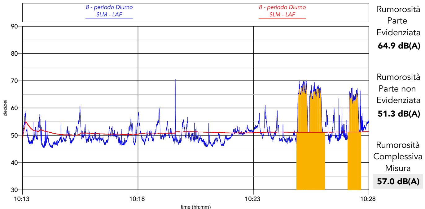
**Percentili complessivi:**  $L_1 = 68.1 \text{ dB(A)}$     $L_{10} = 58.5 \text{ dB(A)}$     $L_{50} = 49.9 \text{ dB(A)}$     $L_{90} = 47.3 \text{ dB(A)}$     $L_{95} = 46.7 \text{ dB(A)}$
