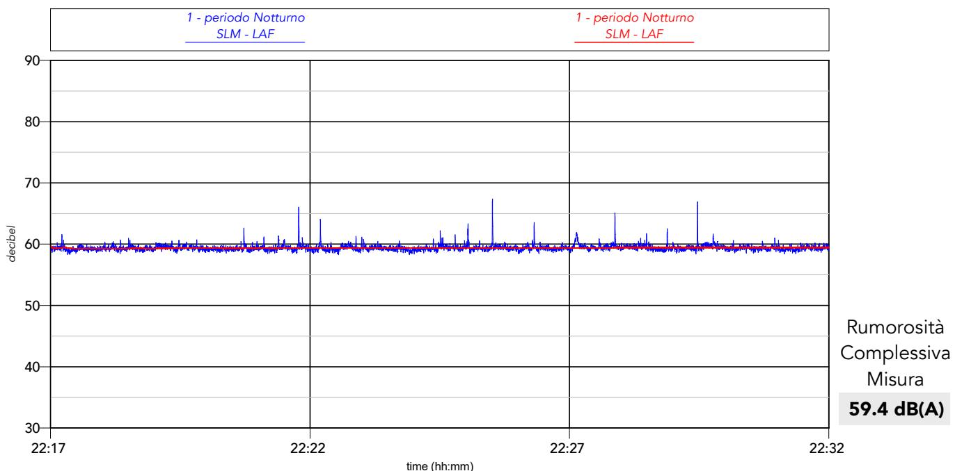
**Percentili complessivi:**  $L_1 = 61.1 \text{ dB(A)}$     $L_{10} = 59.9 \text{ dB(A)}$     $L_{50} = 59.3 \text{ dB(A)}$     $L_{90} = 58.9 \text{ dB(A)}$     $L_{95} = 58.8 \text{ dB(A)}$
