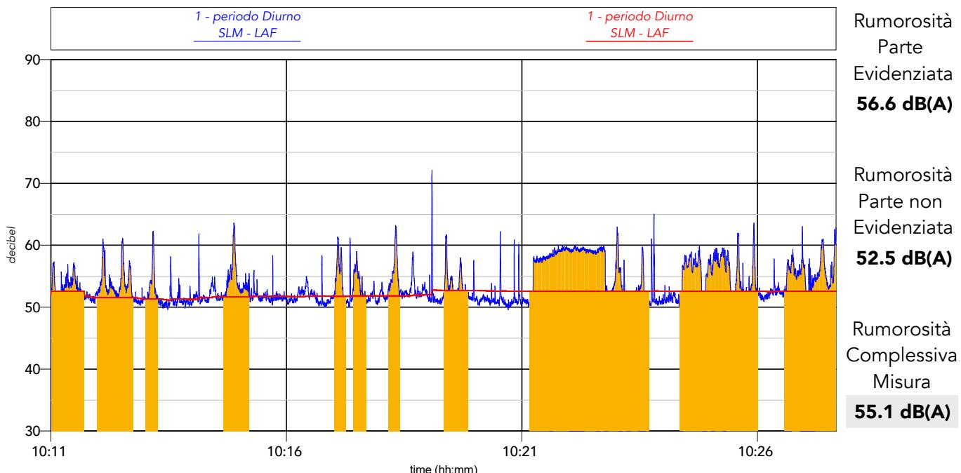
**Percentili complessivi:**  $L_1 = 62.1 \text{ dB(A)}$     $L_{10} = 58.8 \text{ dB(A)}$     $L_{50} = 52.4 \text{ dB(A)}$     $L_{90} = 50.8 \text{ dB(A)}$     $L_{95} = 50.6 \text{ dB(A)}$
