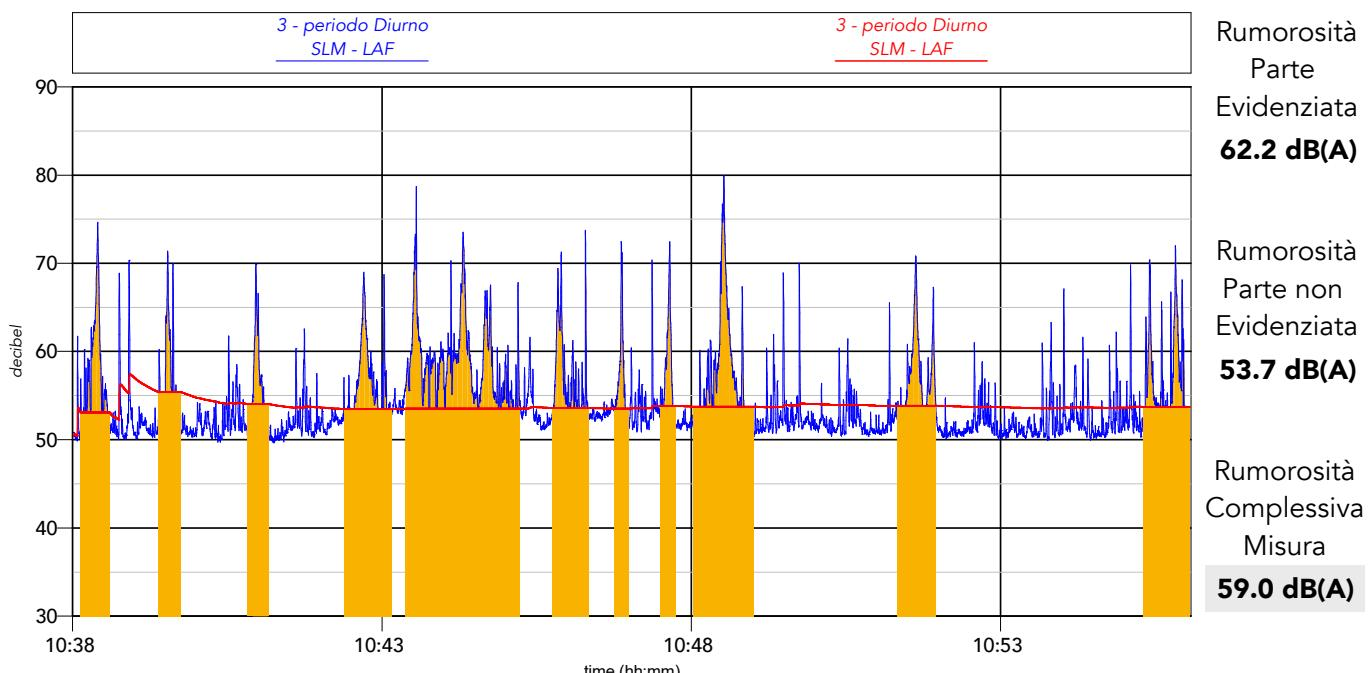
**Percentili complessivi:**  $L_1 = 70.8 \text{ dB(A)}$     $L_{10} = 60.3 \text{ dB(A)}$     $L_{50} = 52.6 \text{ dB(A)}$     $L_{90} = 50.7 \text{ dB(A)}$     $L_{95} = 50.5 \text{ dB(A)}$
