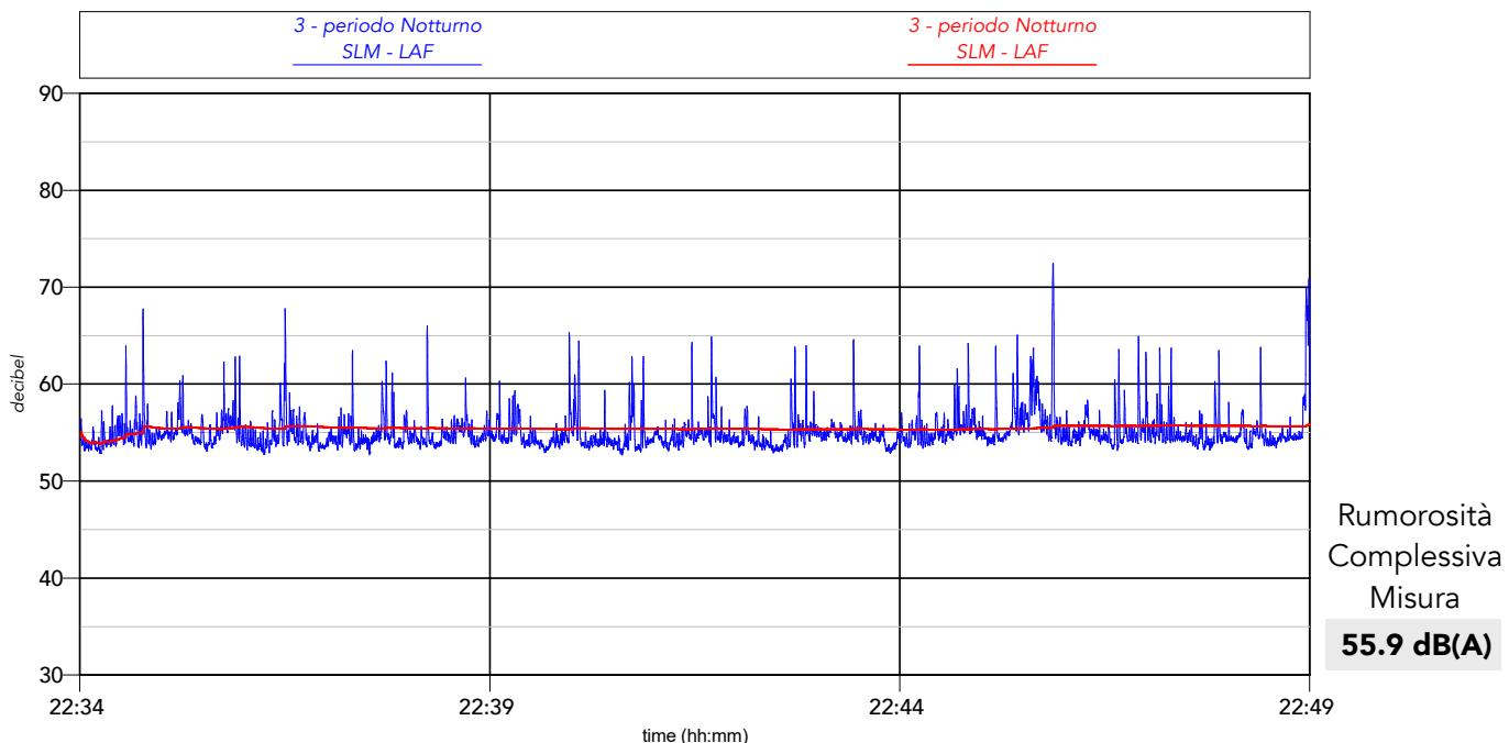
**Percentili complessivi:**  $L_1 = 63.6 \text{ dB(A)}$     $L_{10} = 56.9 \text{ dB(A)}$     $L_{50} = 54.6 \text{ dB(A)}$     $L_{90} = 53.6 \text{ dB(A)}$     $L_{95} = 53.4 \text{ dB(A)}$
