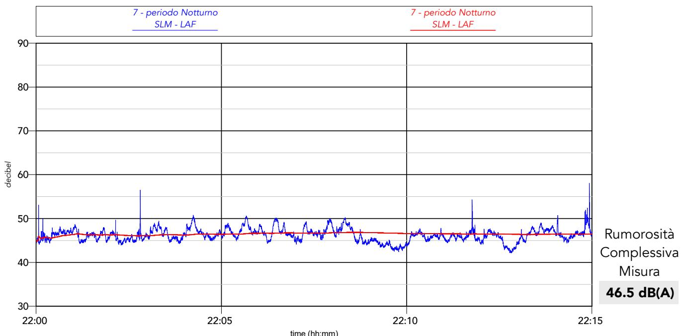
**Percentili complessivi:**  $L_1 = 50.1 \text{ dB(A)}$     $L_{10} = 48.1 \text{ dB(A)}$     $L_{50} = 46.2 \text{ dB(A)}$     $L_{90} = 44.5 \text{ dB(A)}$     $L_{95} = 43.7 \text{ dB(A)}$
