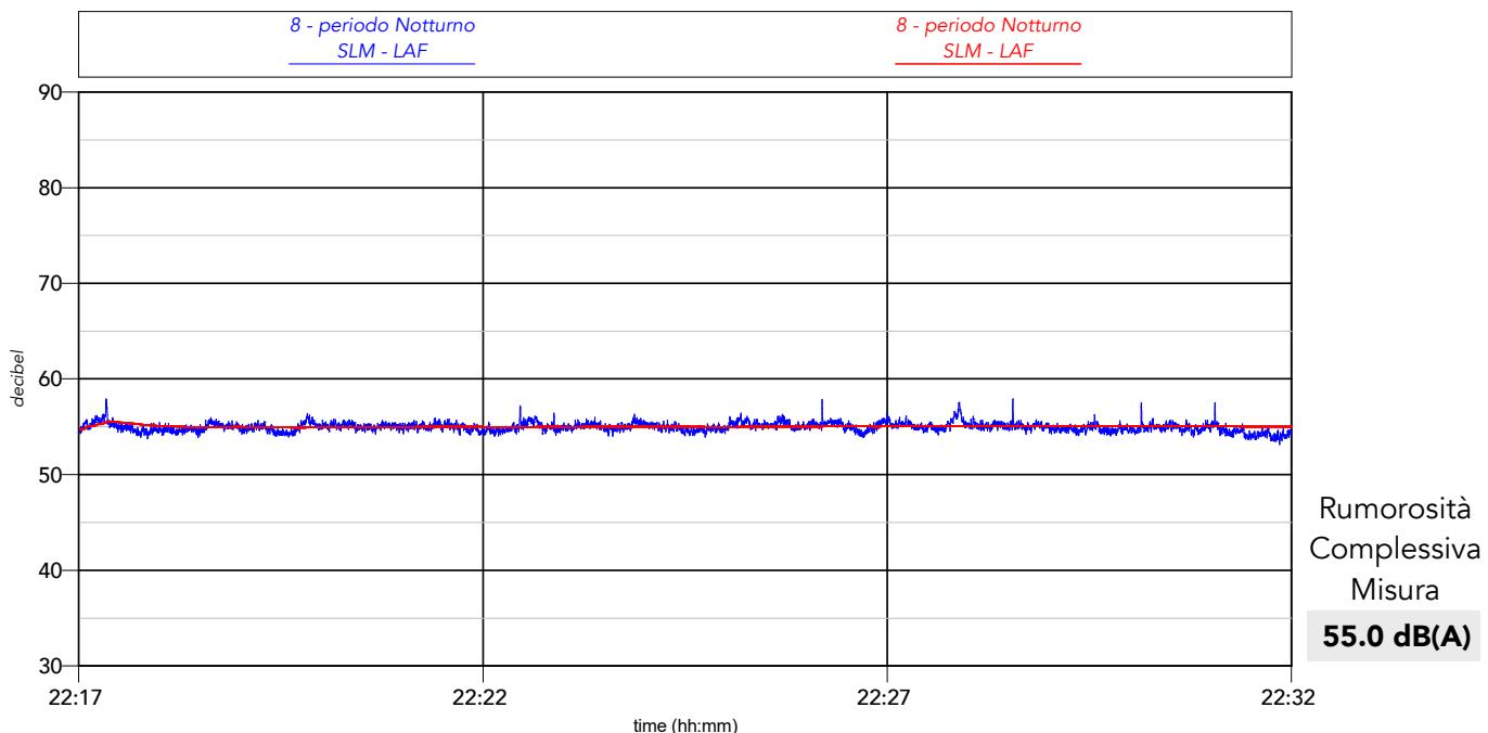
**Percentili complessivi:**  $L_1 = 56.3 \text{ dB(A)}$     $L_{10} = 55.5 \text{ dB(A)}$     $L_{50} = 55.0 \text{ dB(A)}$     $L_{90} = 54.4 \text{ dB(A)}$     $L_{95} = 54.2 \text{ dB(A)}$
