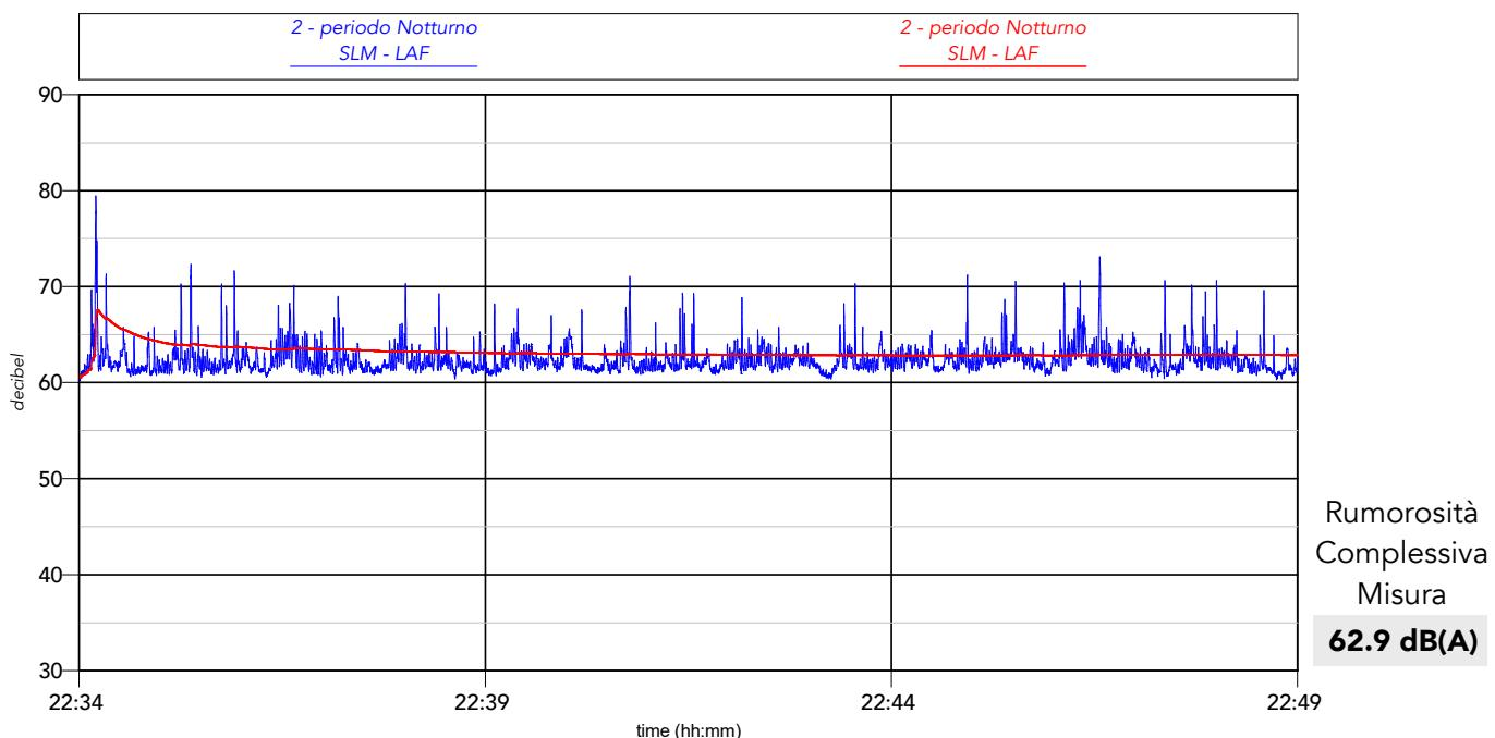
**Percentili complessivi:**  $L_1 = 69.0 \text{ dB(A)}$     $L_{10} = 64.0 \text{ dB(A)}$     $L_{50} = 62.1 \text{ dB(A)}$     $L_{90} = 61.2 \text{ dB(A)}$     $L_{95} = 61.0 \text{ dB(A)}$
