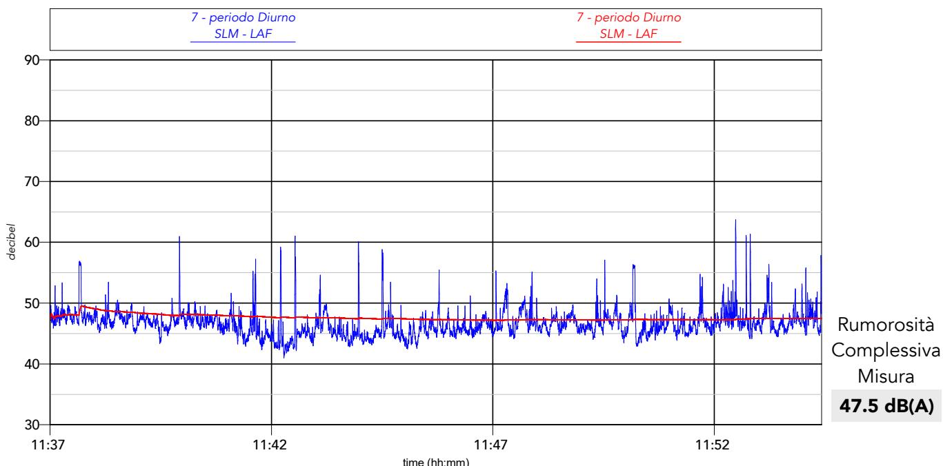
**Percentili complessivi:**  $L_1 = 56.0 \text{ dB(A)}$      $L_{10} = 48.8 \text{ dB(A)}$      $L_{50} = 46.4 \text{ dB(A)}$      $L_{90} = 44.4 \text{ dB(A)}$      $L_{95} = 43.7 \text{ dB(A)}$
